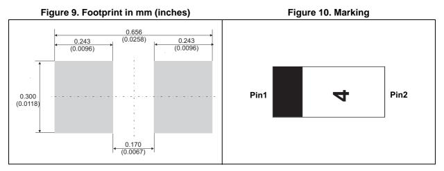
Note: The marking codes can be rotated by 90° or 180° to differentiate assembly location. In no case should this product marking be used to orient the component for its placement on a PCB. Only pin 1 mark is to be used for this purpose.
