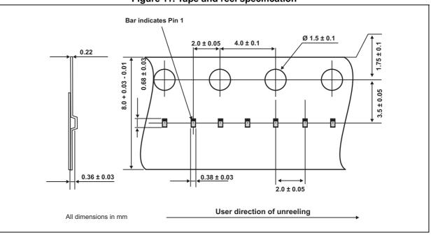
Figure 11. Tape and reel specification
