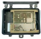
3) Connect cable glands (PGLAND750) or <sup>3</sup>/<sub>4</sub> NPT conduit piping to the face of the midspan. Ensure that connectors are fully installed to guarantee waterproof operation.
