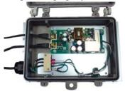
Reattach the protective covering over the PC board and terminal blocks and re-close the lid. Ensure that the four captive screws are fully tightened before operation can commence.
